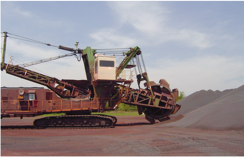
Figure 3. One of three 40 year old 4000 tph bucket wheel reclaimers upgraded by BNSF with three motorised pulleys (one on boom and two on tail.)
