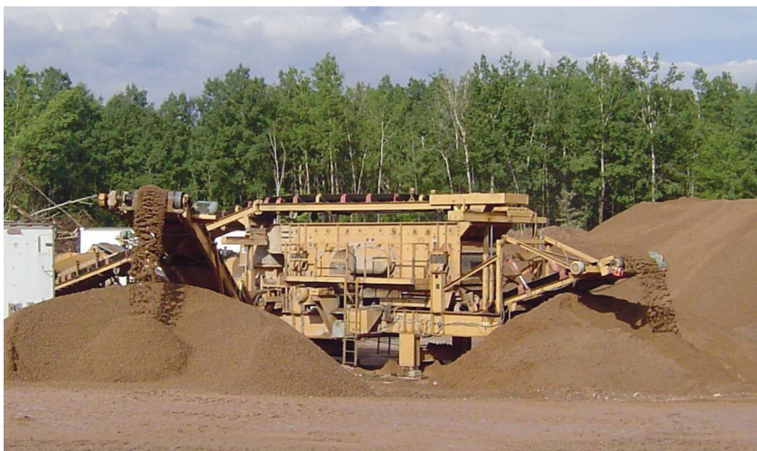
Figure 2. Overview of 800 tph portable recirculating crushing/screening plant which incorporated compact dual 15 hp. motorised pulleys to drive the screen feed conveyor.
