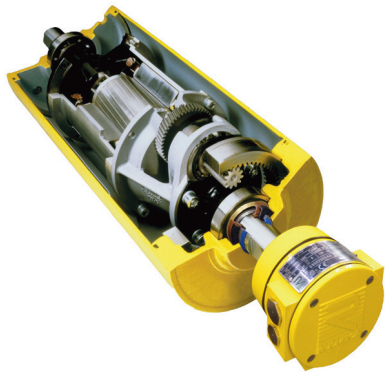
Figure 1. Motorised pulley seals motor and gearbox within oil-filled pulley shell.
